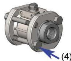
4. Grasp center section by handle or bracket, push back each flange and lift center section clear.
