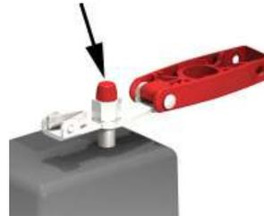
To reengage the drive train, release the override button and turn the handle until the manual override button 'clicks' signaling the re-engagement of the drive train. The manual override lever handle can then be closed.
