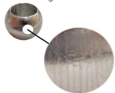
**NOTE:** Prior to disassembly of the Center Section for repair a Valve Repair Kit (VRK89) is required. Kits are supplied based upon valve port size. Each kit contains: (2) Body Seals, (2) Ball Seats, (1) Stem Seal and, (1) Thrustwasher. These are all of the seals contained within the valve. In some cases replacement of the ball may also be required, see Instruction 7.
