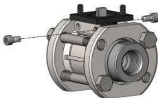
If using a new replacement center section ensure that the drive key is in the same position, i.e. opened / closed, as that of the center section being replaced.
