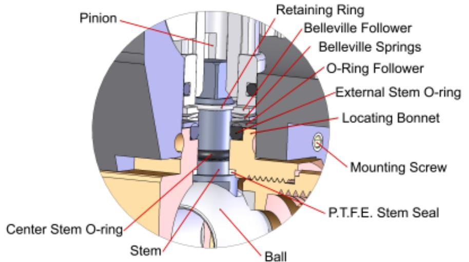
expand radially and maintain contact with the stem.
