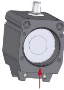
2. Remove and discard the o-ring now visible in the end gland. Replace with new A90126-BU-00 o-ring that was supplied with the kit. Wipe a 1" diameter area around each 1/8" NPT ports.
