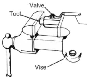
2. Break insert loose by turning tool with a wrench while holding valve body with a second wrench. Remove valve from vise, unscrew insert, remove seat from insert and discard.
